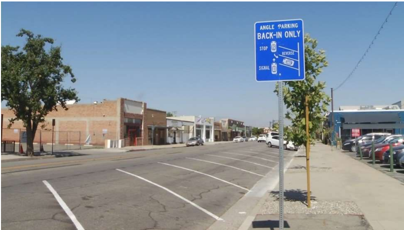
Figure 41. Back-in angle parking signage
