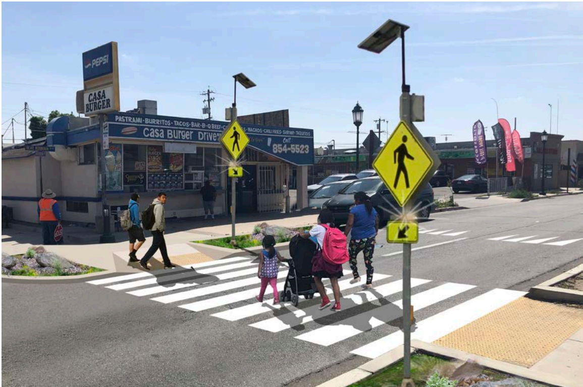
Recommended improvements to Bear Mountain Boulevard include marked crosswalks at all intersections and pedestrian-activated flashing beacons.
