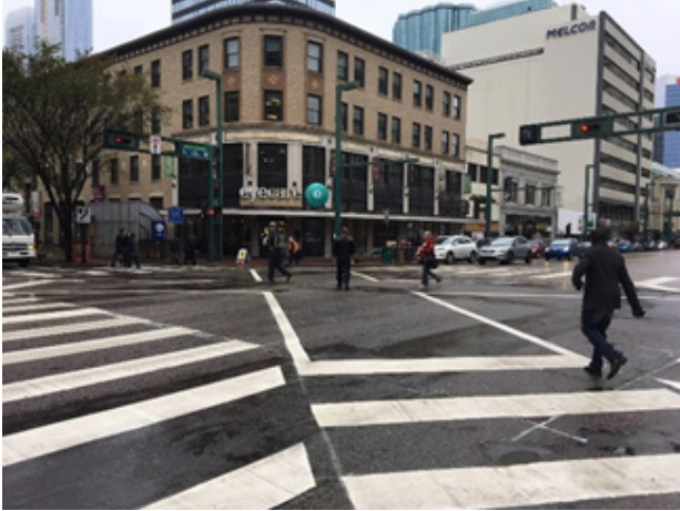
All Way Pedestrian Crossing Phase (Scramble Crosswalks)
