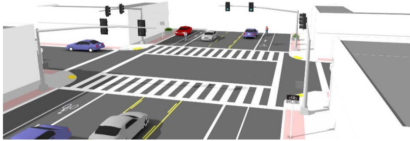
Ladder and transverse crosswalk markings
