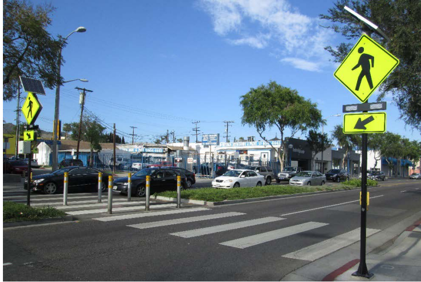
Rectangular rapid flashing beacon
