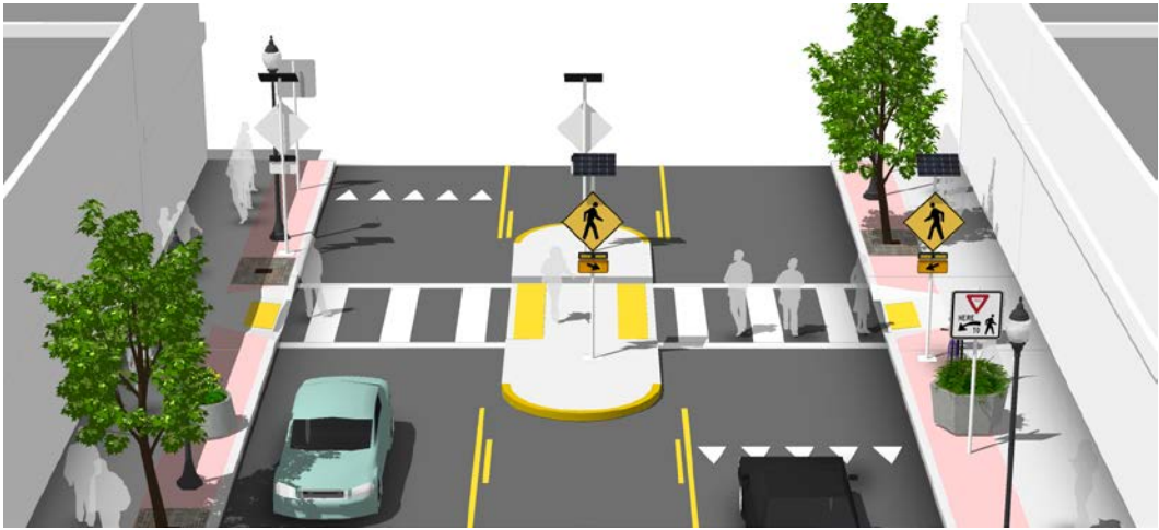
Rectangular Rapid Flashing Beacon with Advance Yield Lines
