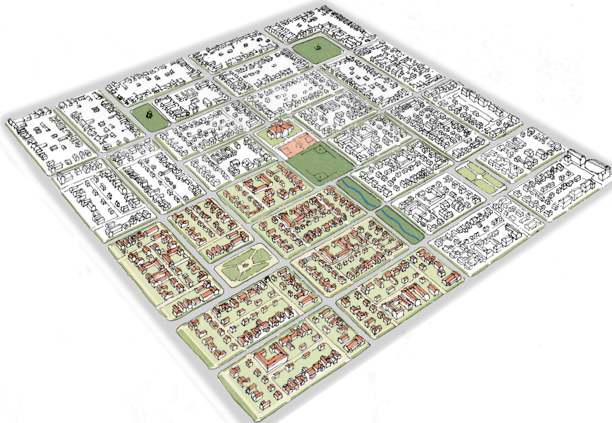
Above: Blocks can be organized into subdivisions composed of an interconnected network of pedestrian-scaled streets and alleys. This diagram illustrates four individual neighborhoods approximately 1200' (1/4 mile) in diameter, made up of about 8 blocks, each with a neighborhood amenity (such as a park) at its center. At the intersection of four such neighborhoods a larger amenity, such as a neighborhood shopping center or school could be located. Using the proposed building types, each neighborhood could accommodate approximately 360 units (900 people) on about 35 acres, or roughly 1500 families (3500 people) on 140 acres.
