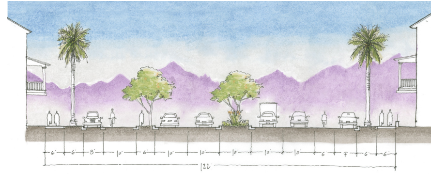
Above: Streets larger than the 100' Four Lane Avenue should be treated with a boulevard section as shown that provides a local access lane designed for very slow speeds and parallel parking.
