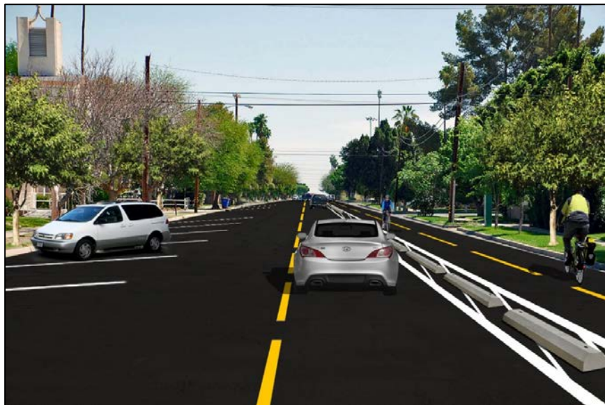
Figure 4-33: Option 7C would provide a two-way cycle track on the south side of Seventh Street
