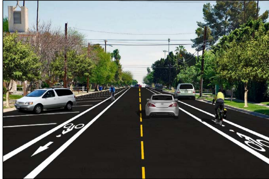
Figure 4-30: Option A for Seventh Street reconfiguration with bike lanes next to travel lanes
