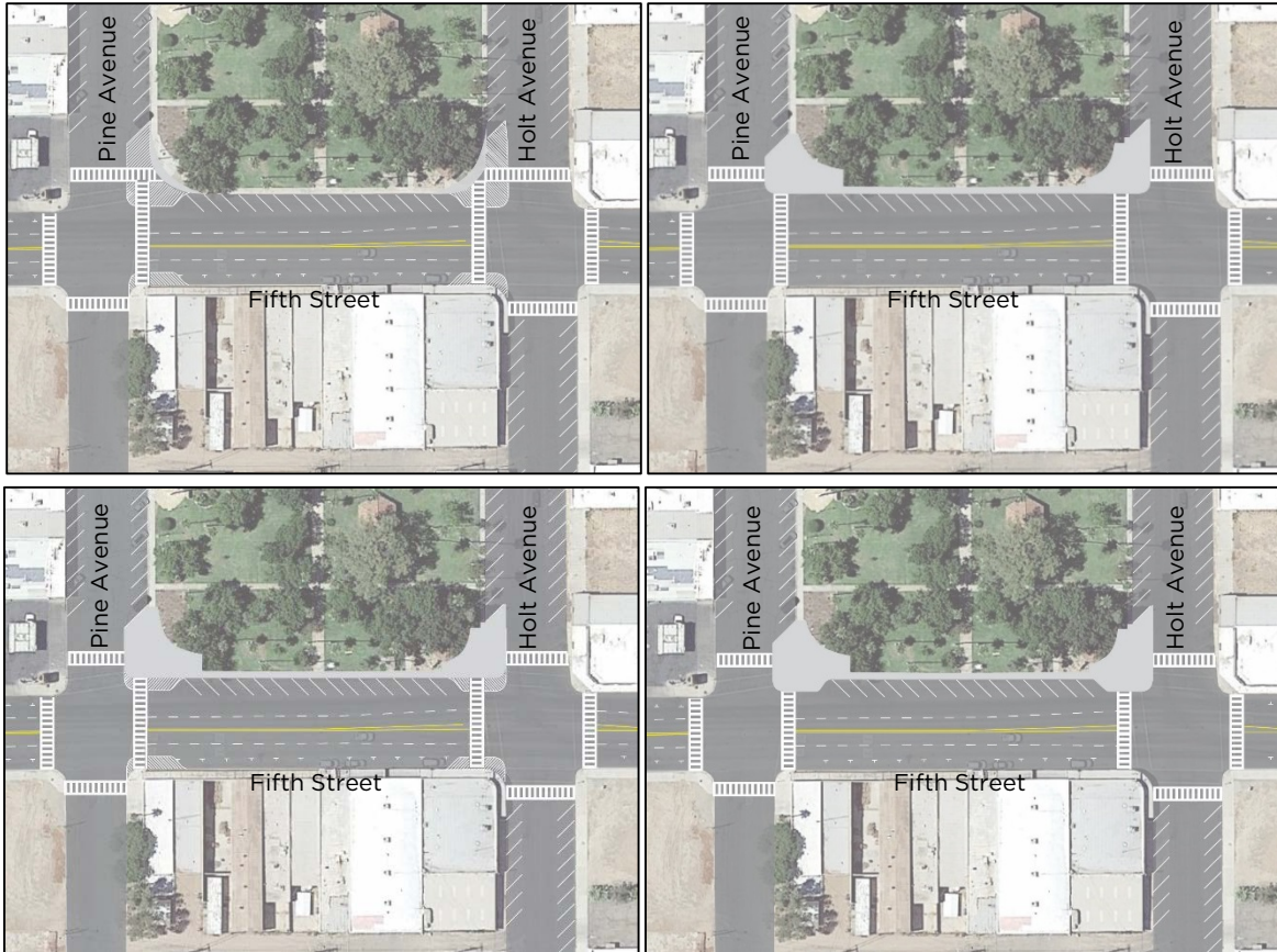
Figure 4-12: Clockwise from top left: painted bulbouts; concrete bulbouts solely in City right-of-way; concrete bulbouts solely in City right-of-way with painted extension with Caltrans right-of-way; and full concrete bulbouts (the ideal solution)
