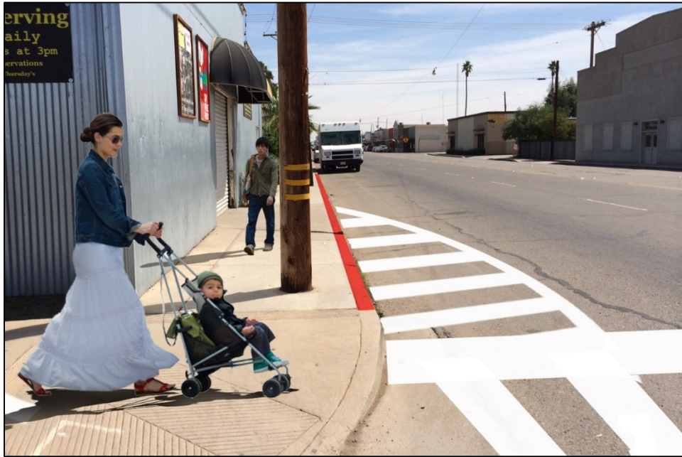
Figure 4-17: Simulation of the northeast corner of Fifth Street and Cedar Avenue with Option 3A - painted crosswalks and bulbouts
