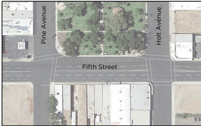
Figure 4-8: Aerial view of Fifth Street at Holt Park. Current crosswalk design does not meet ADA or Caltrans standards
