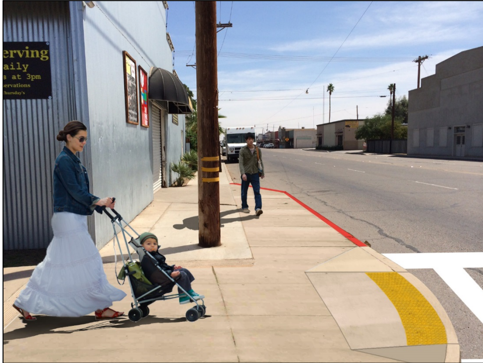
Figure 4-19: Simulation of Option 3B with permanent bulbouts to reduce crossing distances and increase sidewalk space for pedestrians
