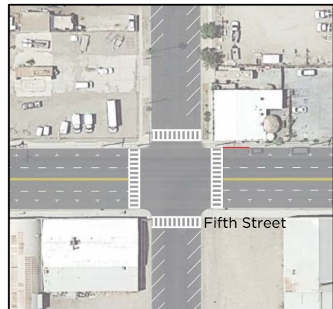
Figure 4-16: Intersection of Fifth Street and Cedar Avenue with continental crosswalks
