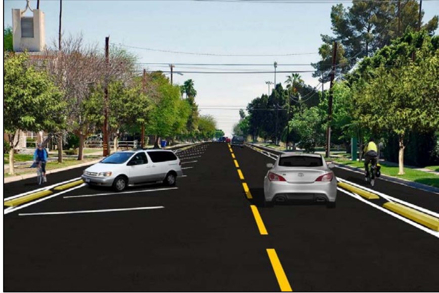
Figure 4-32: Option 7B for Seventh Street reconfiguration with bike lanes next to the sidewalks
