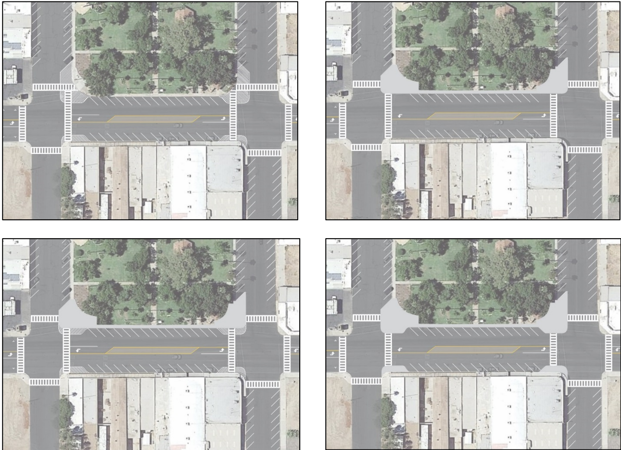
Figure 6-10: Fifth Street after road rightsizing. Clockwise from top left: painted bulbouts; concrete bulbouts solely within City right-of-way; concrete bulbouts solely within City right-of-way with painted bulbouts beyond; and concrete bulbouts
