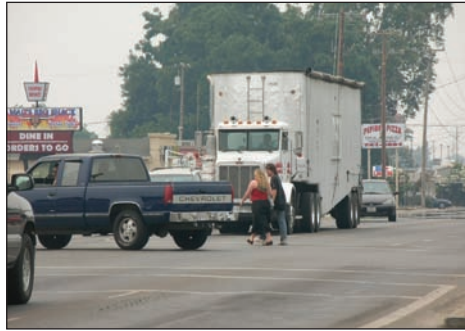
Left: Lack of separation between turning and through lane and location and size of driveway creates hazardous conflicts for motorists and non-motorists alike; right: pedestrians make perilous crossing.
