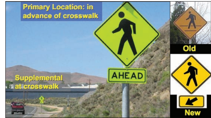
New MUTCD standards specify the sign design shown above for placement in advance of pedestrian crossings. A directional arrow (shown on the right) is specified for signs located at the crosswalk.
