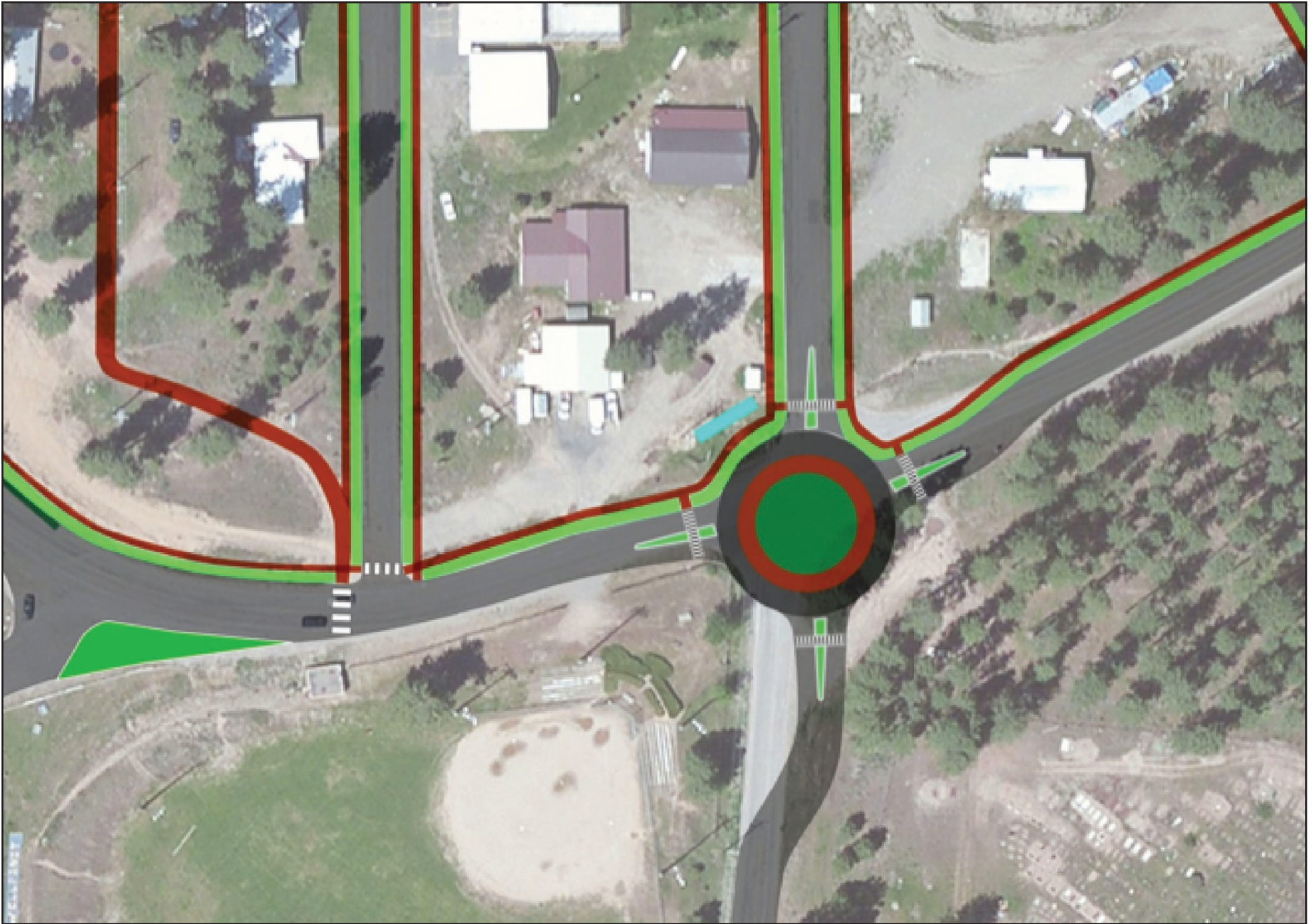
Figure 6. Diagram of roundabout at BIA Highway 27/Wellpinit Agency Loop/Ford-Wellpinit Road. The roundabout is characterized by yield controlled entry points, channelized approaches, truck apron for larger vehicles, and high-visibility crosswalks.
