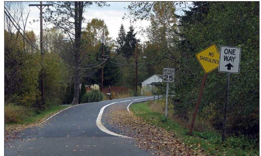
In addition to striping, signage is crucial to the success and safety of a Scenic Slow Road
