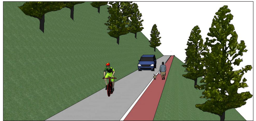
Where the travel way is limited to one lane, bicycles can use the roadway while pedestrians can safely use the shoulders
