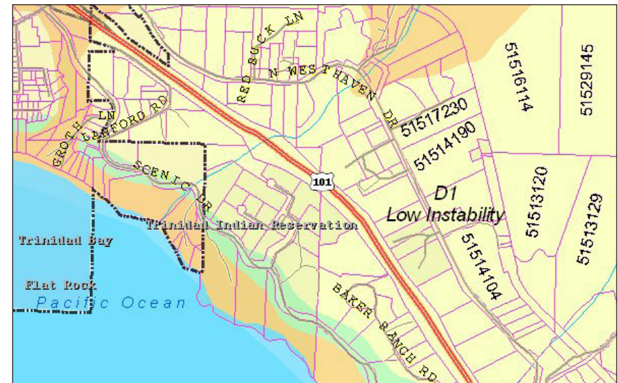
Coastal sections along Scenic Drive & upper reaches of McConnahas Mill Creek are areas of high geologic instability – Humboldt County GIS
