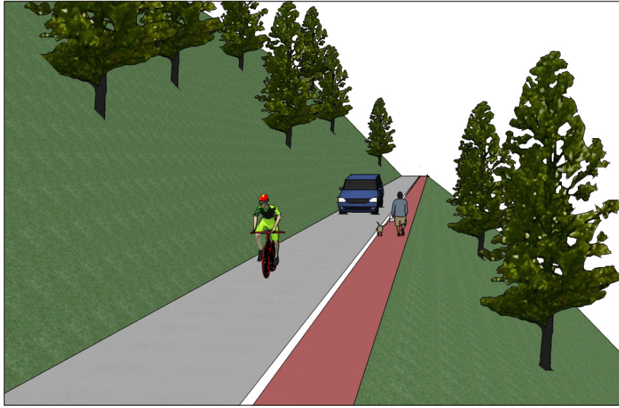
Where the travel way is limited to one lane, bicycles can use the roadway while pedestrians can safely use the shoulders
