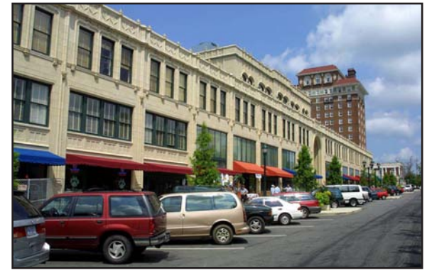
Head-in angled parking is familiar to most motorists along with its primary benefit (larger parking supply) and its primary safety problem (blindly backing out into a travel lane). A growing number of cities are converting their head-in parking to back-in parking.
