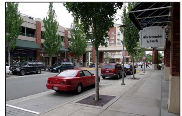
Head-in angled parking is familiar to most motorists along with its primary benefit (larger parking supply) and its primary safety problem (blindly backing out into a travel lane). A growing number of cities are converting their head-in parking to back-in parking.
