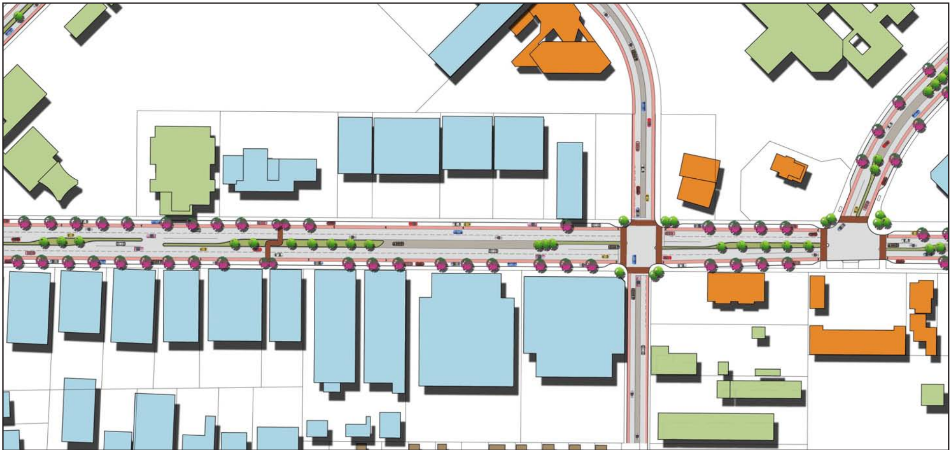
Figure 3-3: North Santa Anita Avenue from City Hall to Tyler Avenue. Note intersection improvements, continuous landscaped median, and mid-block pedestrian crossing.
