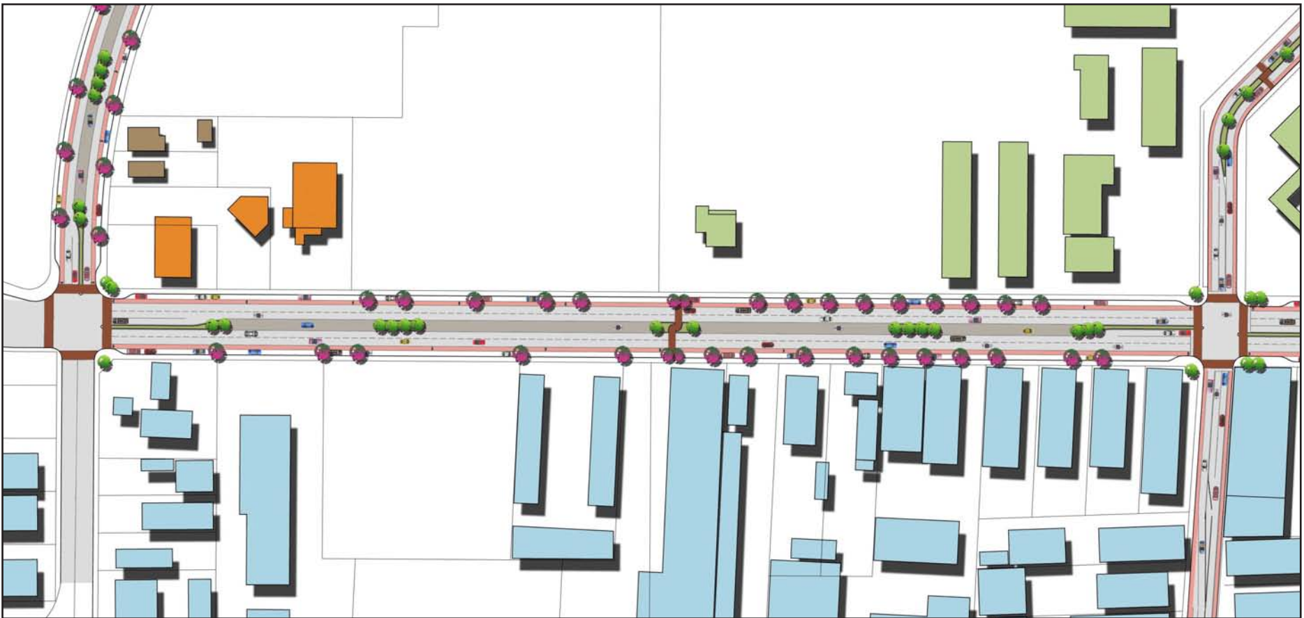
Figure 3-2: North Santa Anita Avenue from Merced to Central. Note intersection improvements, intermittent landscaped median islands, and mid-block pedestrian crossing.
