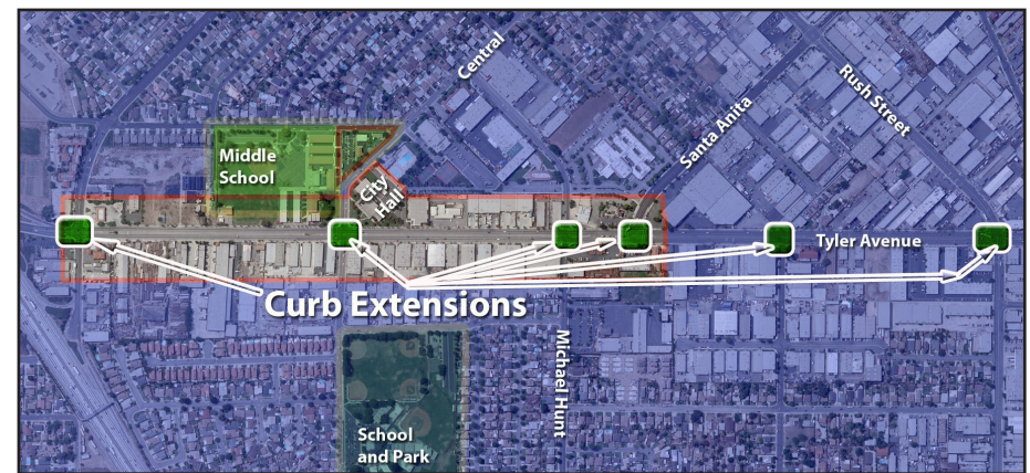
Figure 3-9: Intersections where curb extensions should be installed
