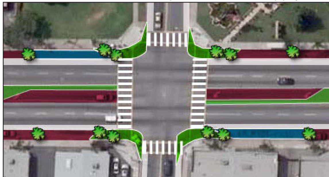
Figure 3-21: Curb extensions and landscaping (green), parking and turn lanes (red), and bus stops (blue).
