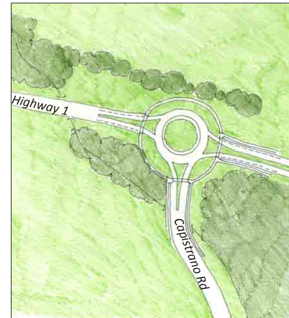
Capistrano Road is shifted south to form a simplified intersection with a roundabout.
