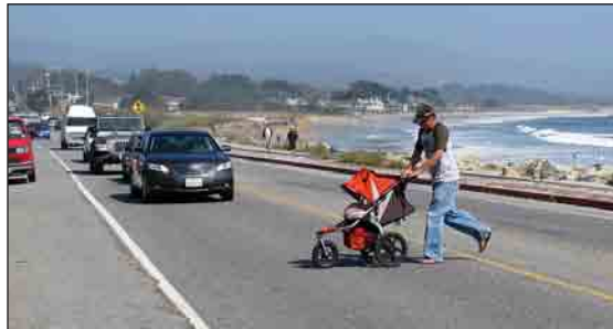
People want and need to cross the highway at convenient locations. Providing well-designed, highly visible crosswalks at convenient locations can help consolidate random crossings. Fences and barriers to force pedestrians to use inconvenient access points can be expensive, unsightly, and futile.
