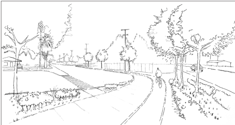
The drawing on the left illustrates the addition of a paved trail parallel to Manning Avenue. Motor vehicle access to Pine Avenue from Manning Avenue is closed, eliminating conflicts between cars and trail users at this location.
