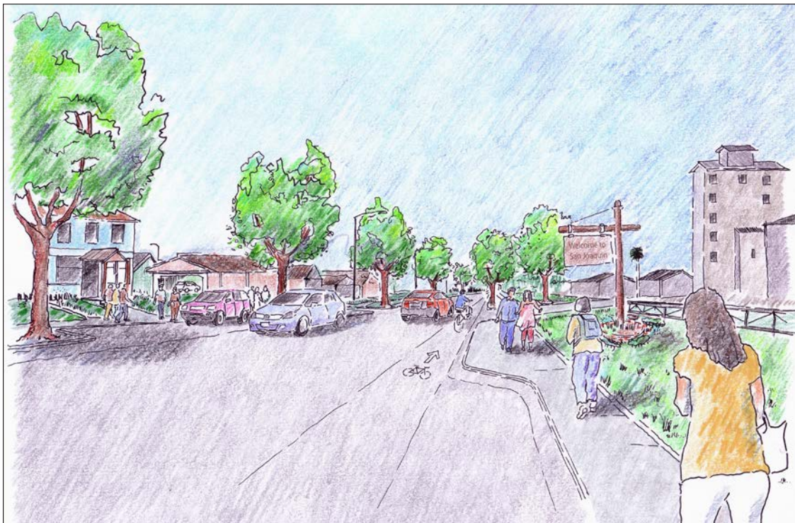
The drawing above shows a long-term concept for Colorado Avenue that would include the addition of a sidewalk and welcome sign and bike lanes on both sides of the roadway.
