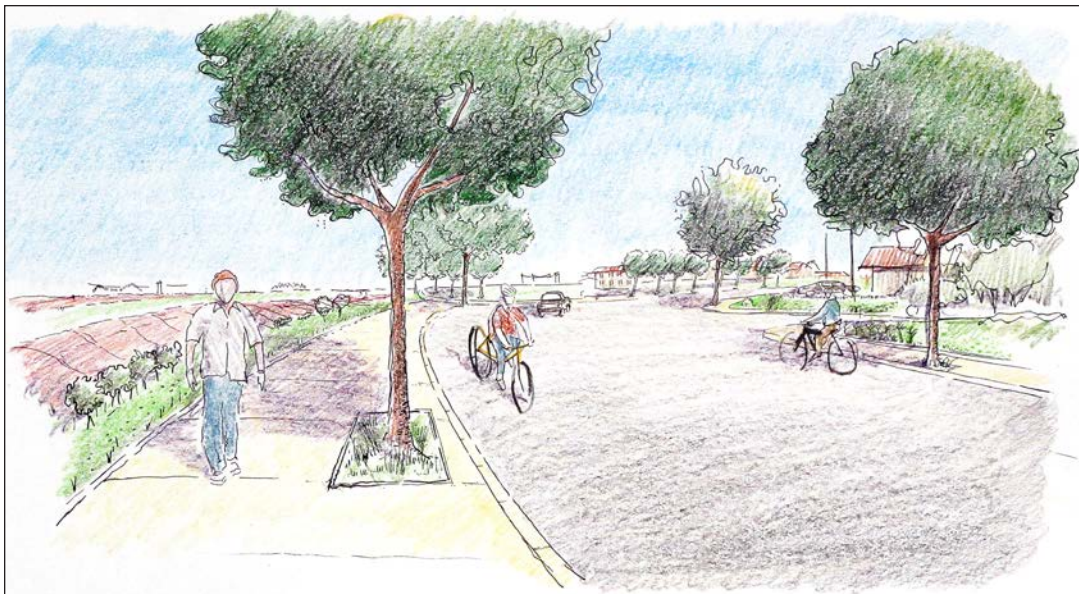
The drawing above illustrates the improvement of Elm Street with a wide tree-planted sidewalk or pedestrian path developed on the north side of the street and bike lanes on both sides of the street.
