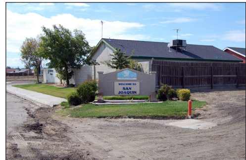
Curbs, sidewalks and other features slow traffic more than speed signs. The start of a vertical curb and gutter, sidewalk, a welcome sign and other elements shown in the photo above alert motorists to the change in context.
