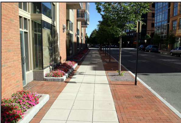
A well designed sidewalk includes a pedestrian zone clear of obstacles.
