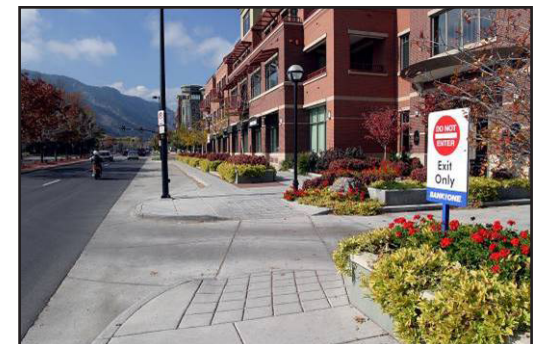
Landscape bumpouts and sensitive ramp treatments can ease driver behavior when frequent driveway cuts need to be employed.
