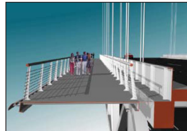
Figure 3. Example of Multi-Use Path Cantilevered off an Existing Bridge Structure. Source: Caltrans
