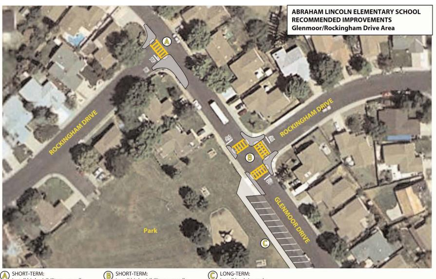
Install high-visibility crosswalk striping and curb ramps
