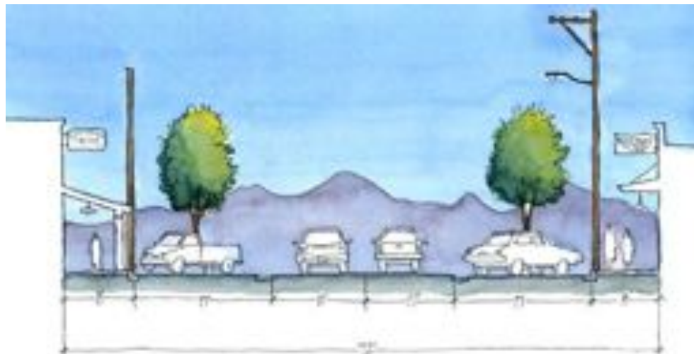
Proposed right-of-way shows two 11' travel lanes, angled on street parking with tree wells every 30'. The existing 56' cross section is suitable for such a configuration which can help calm traffic in the downtown and better service existing businesses; potential vehicle/bicycle conflicts can be mitigated if Class III facilities are implemented along Main.*
