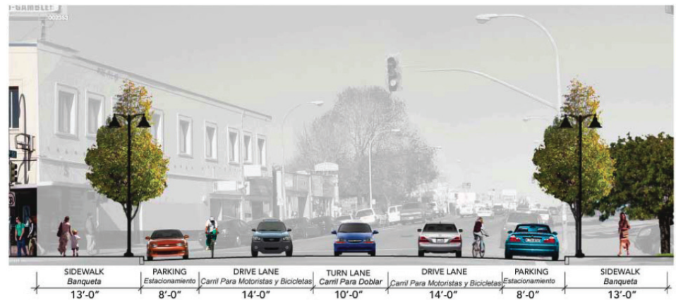
The diagram shows the proposed cross section for 23rd Street looking north from Macdonald Avenue. Streetscape concept by Callander Associates Landscape Architecture, Inc.
