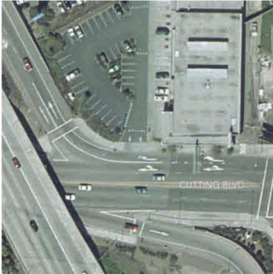
The 2 lane on-ramp, broad, sweeping corner and crosswalk placement forces pedestrians to follow indirect route across 2 lanes of accelerating traffic.
