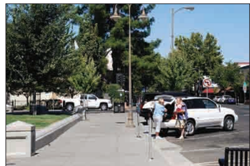
Back-in angled parking provides safe unloading for child and stroller at park in Chico, Ca.
