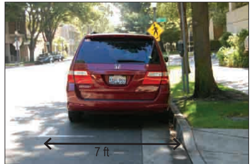
Top and Above: 7-foot marked parking encourages the car in the bottom photo to park close to the curb.
