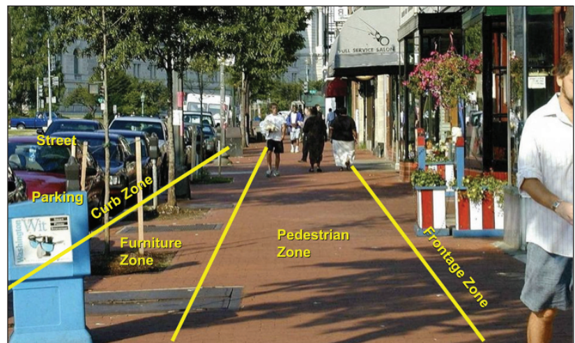
The upper and lower images show the arrangement of sidewalk corridor zones on residential and commercial and mixed use streets.
