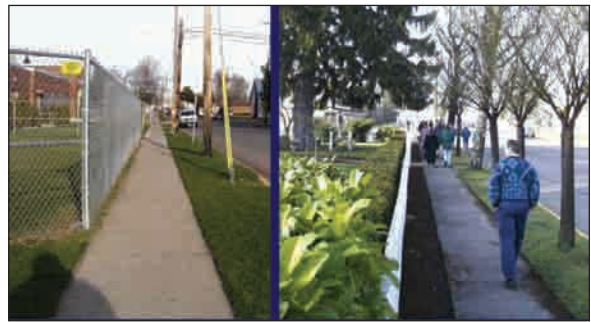
The type of fence material impacts pedestrian comfort: the sidewalk on the left is wider, but feels constrained because of a high chain link fence.
