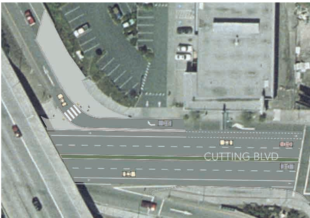
The diagram illustrates changes to Cutting Boulevard and the I-80 northbound on-ramp enabling pedestrians to cross one vehicle lane prior to vehicle acceleration. Space on Cutting is also reallocated for a bike lane with reduced area of conflict between bicyclists and vehicles merging to the on-ramp.
