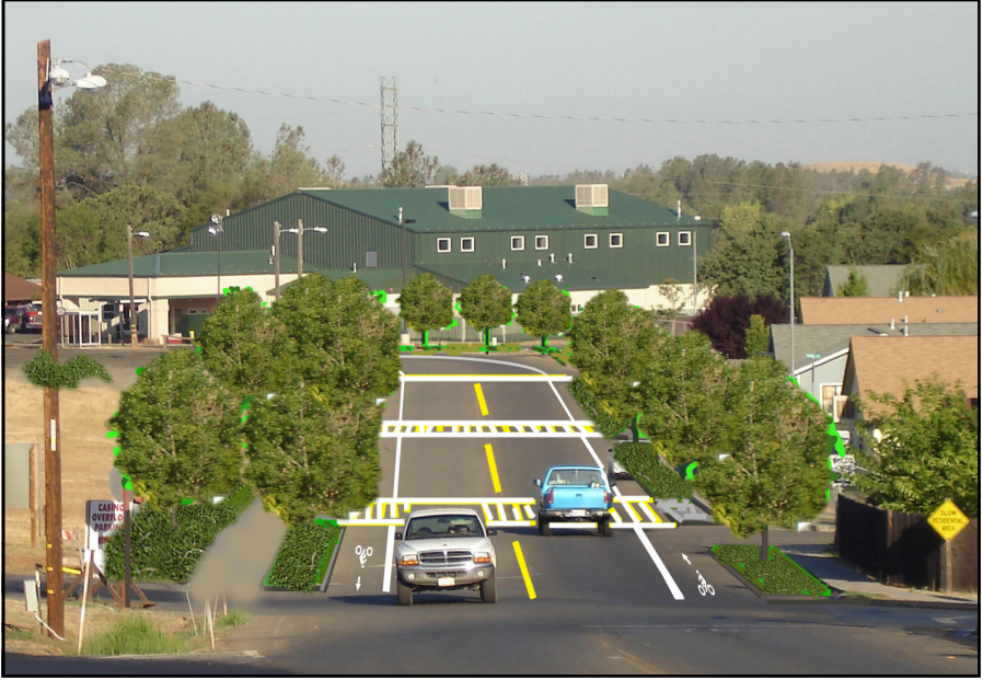
Figure 3. Traffic Calming on Alverda Drive Photo montage shows what Alverda Drive would look like with sidewalks, trees, narrower lanes and marked crosswalks.
