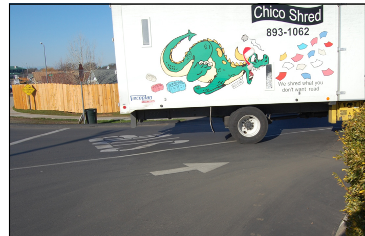
Due to the skew of the intersection at Alverda Drive and Feather Falls Boulevard, larger vehicles need to travel in the opposite lane at this entrance to the Casino.
