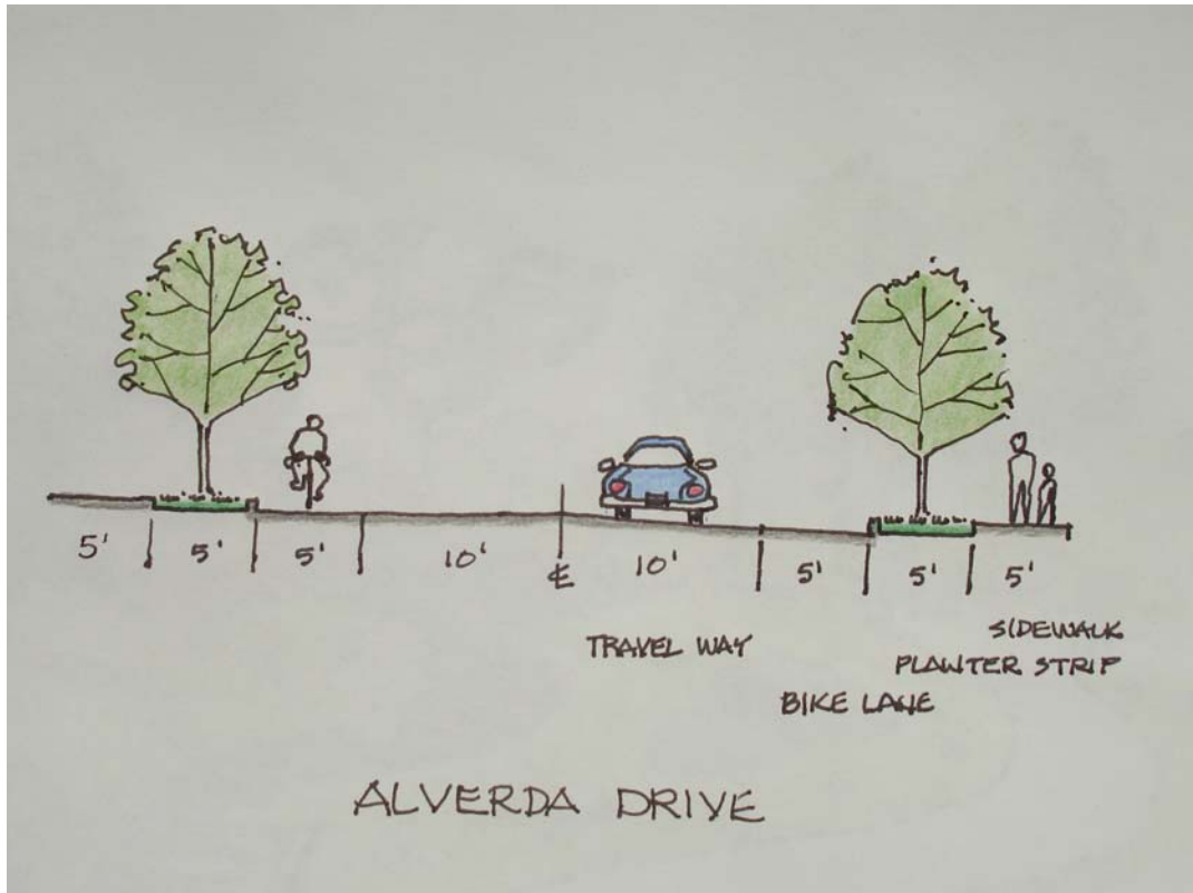
Figure 3. Typical Section through Alverda Drive
