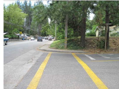
A standard marked crosswalk with two parallel stripes – standard crosswalks are appropriate at stop or signal-controlled locations
