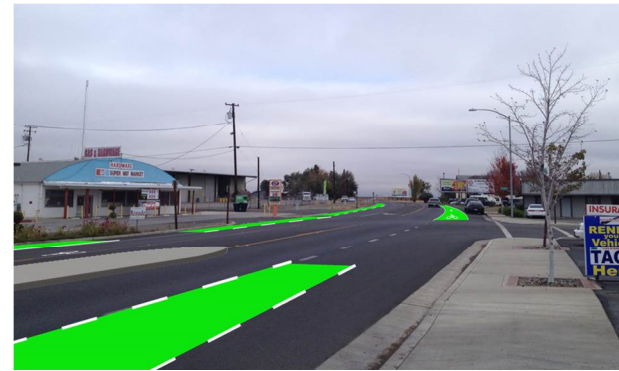
Phase 1 Improvements – Green Bicycle Lanes and Raised Median
