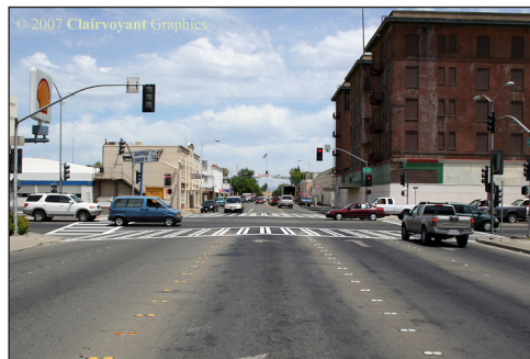
High-contrast, ladder-style crosswalk markings are much more visible to motorists, as shown above. The top photo is the existing intersection, while the bottom is a simulation.
