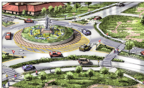
The roundabout in the illustration is under construction in Reno, NV. Note how single and dual lanes are combined with right-turn slip lanes.
