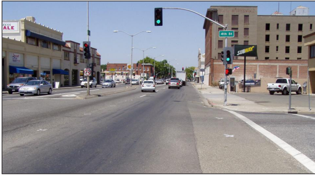
The motorist's view of the same intersection and simulated crosswalk markings. High-contrast markings alert drivers to watch out for pedestrians. Ladder-style markings are spaced so that vehicle tires travel between crossbars, instead of over them. This reduces wear and maintenance of crosswalk markings.
