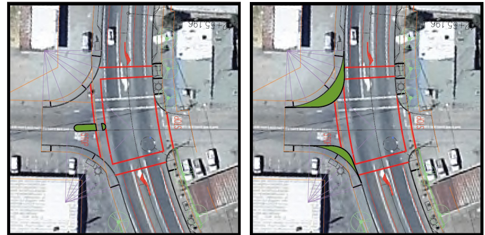
Figure Figures 5-4, 5-5, and 5-6 illustrate the potential for a roundabout at the intersection of Highway 101 and Branscomb/Dos Rios Road.
