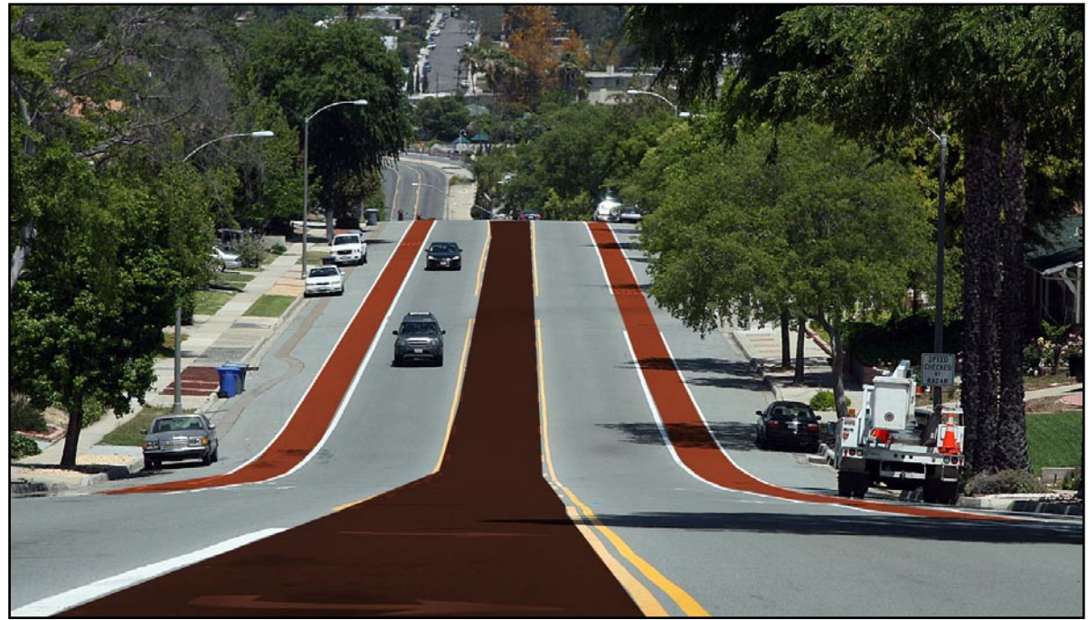
Figure 3-26: Suggestion for Severin Drive with colored bike lanes, and landscaping to narrow driver's space.
