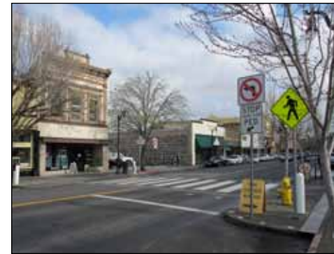
High-visibility longitudinal bars and signage draw attention to a mid-block crossing.
