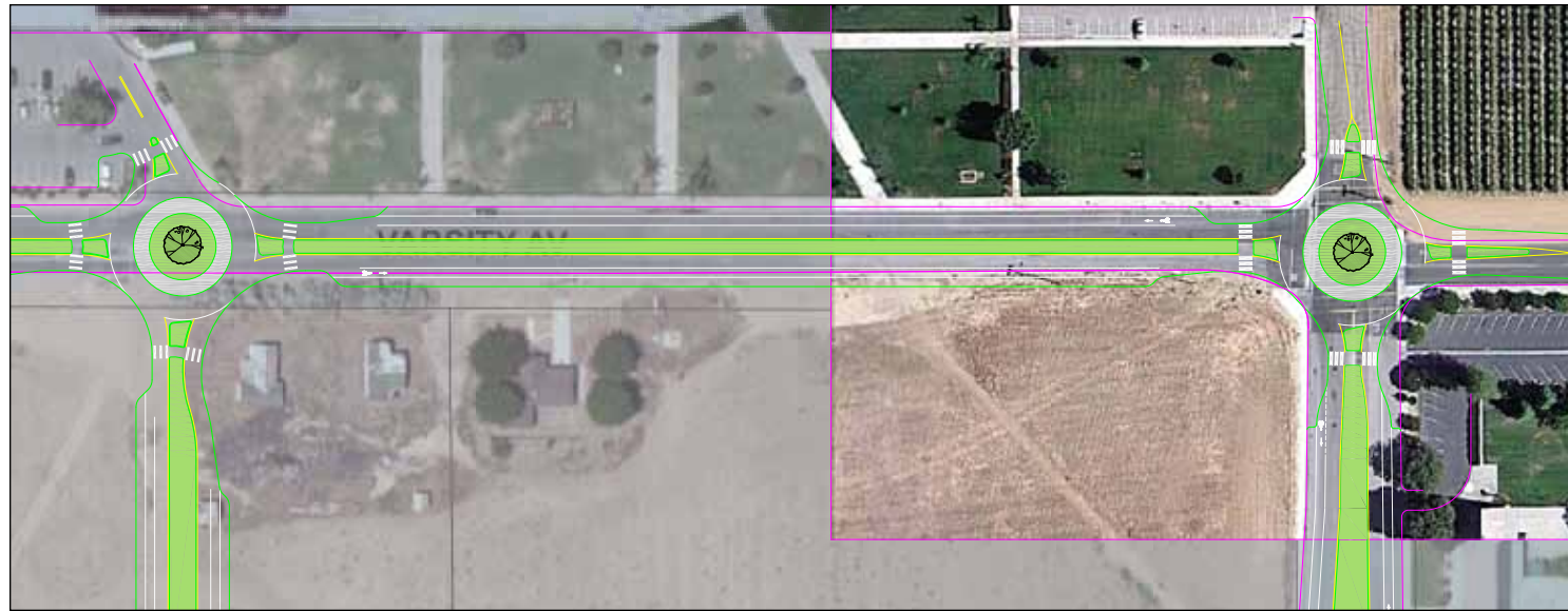
Caption: Varsity Road provides access to Arvin High School and will connect to the Walnut Drive extension once completed. Today the southern edge of Varsity along Jewett Square is unimproved. Varsity can be developed as a 2-lane roadway with Class II bike lanes, on-street parallel parking, and sidewalks on either side. Roundabouts at the intersections of Walnut Drive and Campus Drive can improve the functionality of these respective intersections and help to facilitate circulation around Arvin High School.
