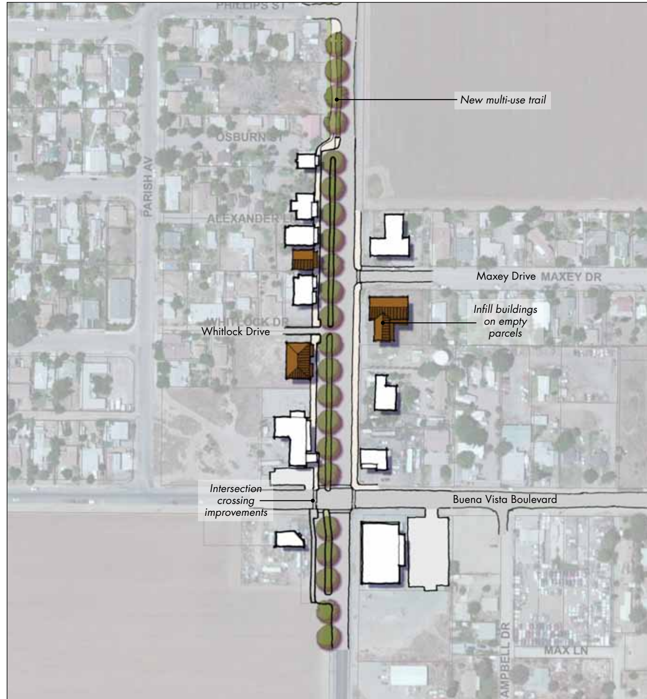
Above: In central Weedpatch, commercial buildings currently maintain an unusually large setback from SR 184, especially on the west side of the road. A frontage road is proposed from Osborn Lane to one half-block south of Buena Vista Boulevard to capitalize on this extra space between the buildings and the highway. No longer competing with the high speeds of Weedpatch Highway, a frontage road would offer a more comfortable main-street environment for residents and local businesses to thrive. Small new commercial buildings are shown ultimately infilling the empty lots on the corridor.
