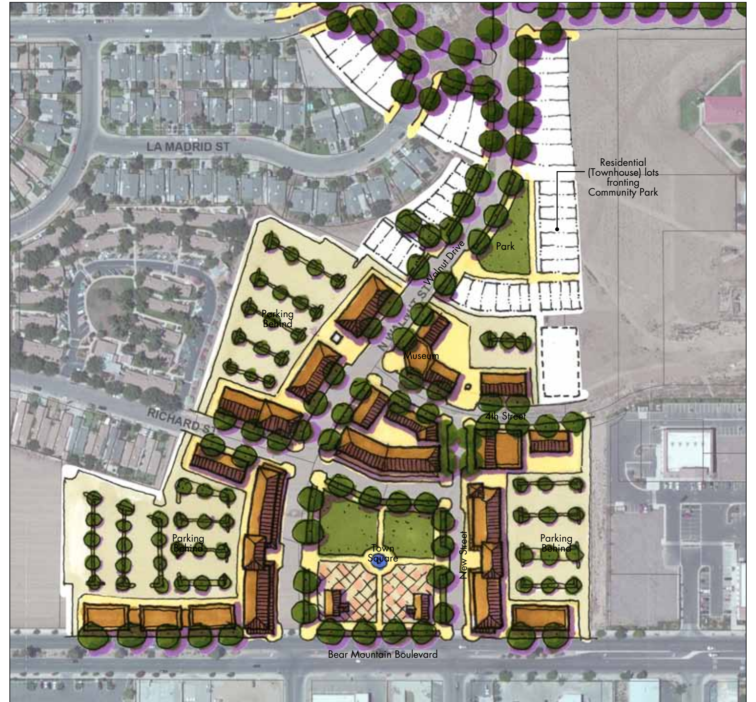
Above: Detailed illustrative plan of the alternative option, demonstrating the continuation of a "Main Street" along Walnut Drive and the relocating of some of the community park elements into the town square.
