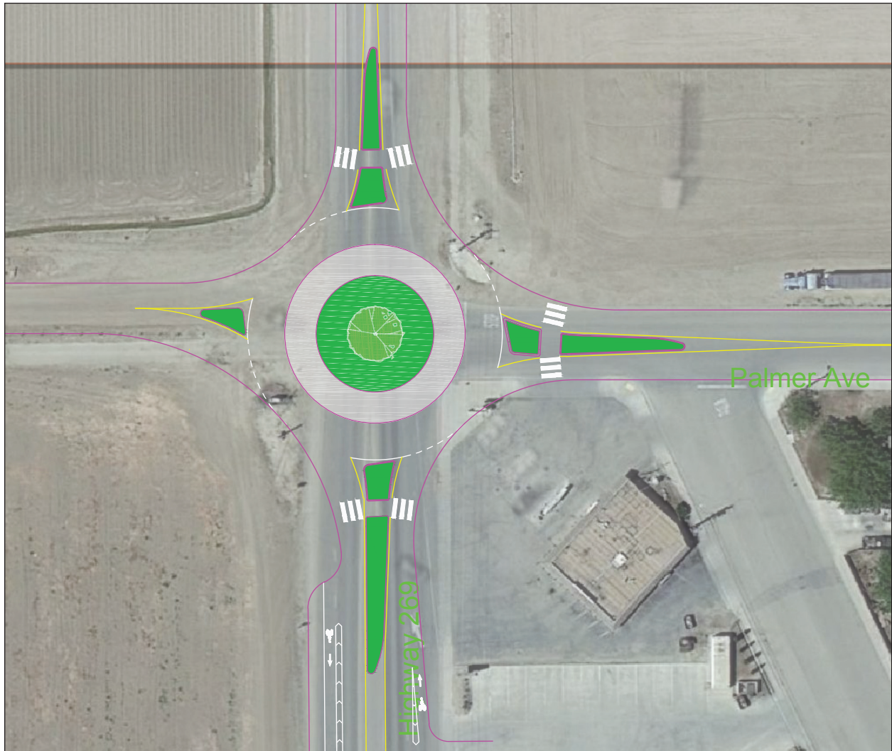
Figure 33. Roundabout design at Lassen Avenue and Palmer Avenue. (Conceptual – Not For Construction) Source: Nelson\Nygaard.
