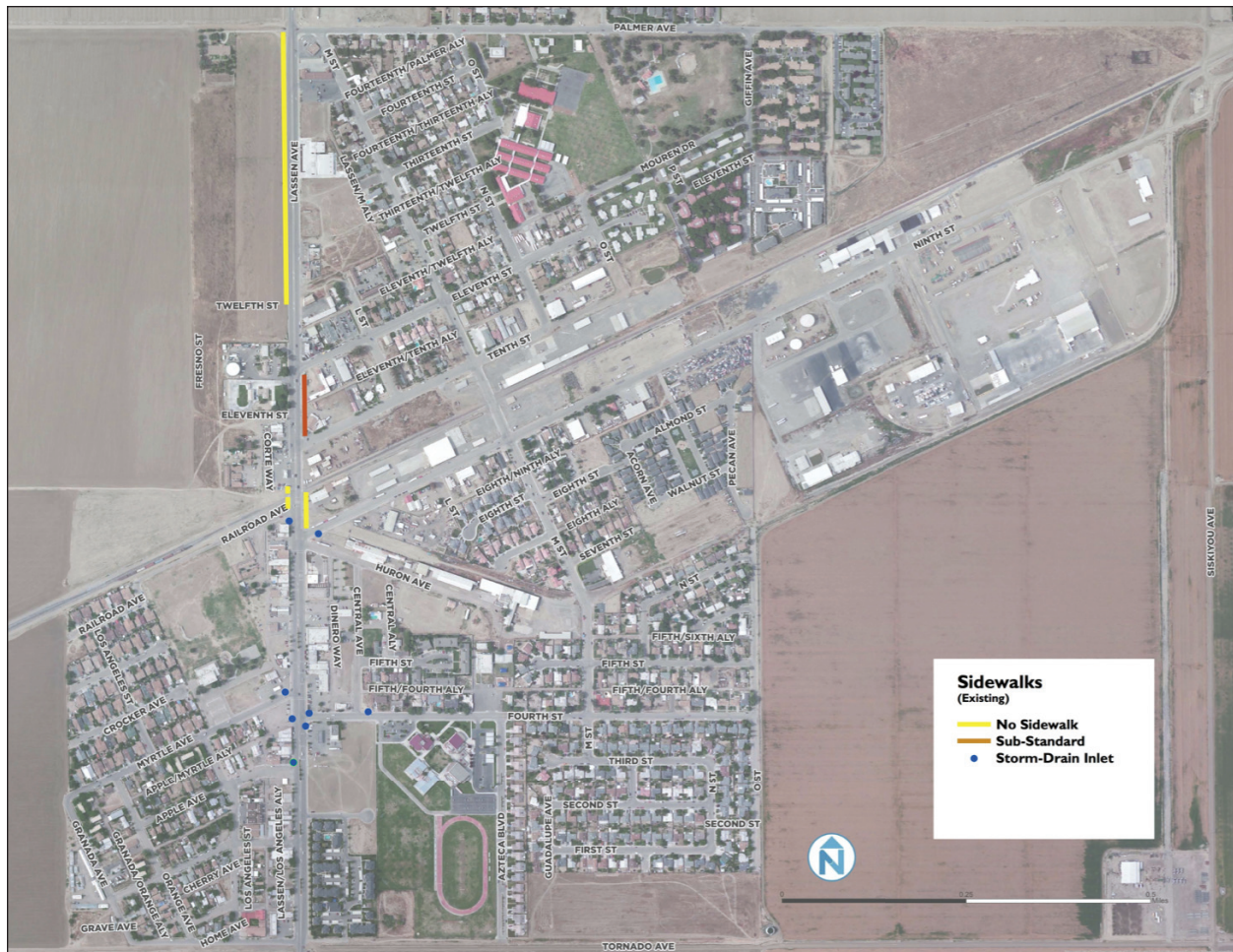
Figure 37. Sidewalk and drainage existing conditions.
