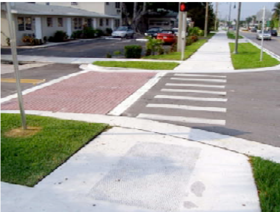
Pedestrian crossing points at driveways can be striped or designated with different materials.
