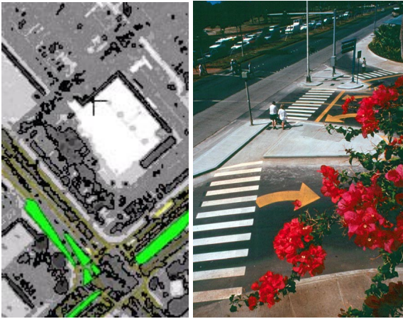
This image of a Honolulu, Hawaii, crossing illustrates the concept for a channelized island at the Kearney Palms Shopping Center entrance.
