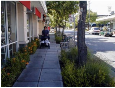
A buffer, or planting strip, between the sidewalk and the curb provides separation between traffic and people who are walking. It also provides space for landscaping and street amenities.
