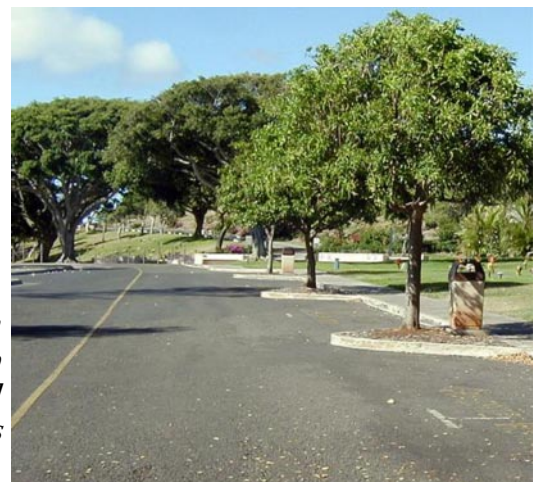
Tree wells, like those shown in the photo at left, are an effective way substitute for continuous planter strips to buffer the sidewalk from traffic, narrow the roadway, and to allow for parking. This location has two parking places between each tree, but there could be more or less.
