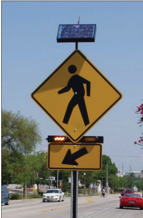
The Rectangular Rapid Flash Beacon (shown above) is not yet in the Manual on Uniform Traffic Control Devices but it has received interim approval from the Federal Highway Administration. These beacons have resulted in much higher yielding rates (approximately 80 to 90 percent) compared to normal circular yellow flashers (approximately 30 to 60 percent, or even lower).
