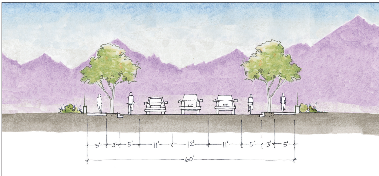
Figure 4.29: Avenue 50 west of Harrison Street – Proposed 60' Segment
