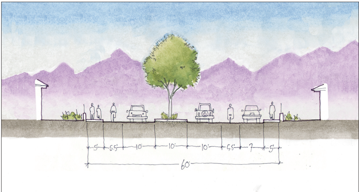
Figure 4.32: Avenue 52 with Curbside Parking — Proposed
