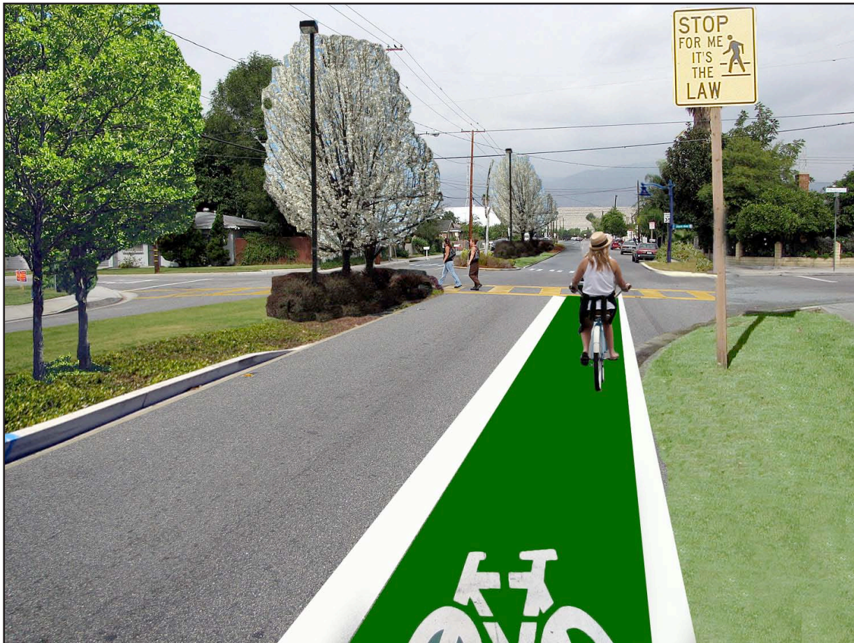
Option for highlighting bicycle lane on Maine Avenue at East Baldwin Avenue.
