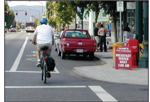
Curb extensions reduce pedestrian crossing distances.
