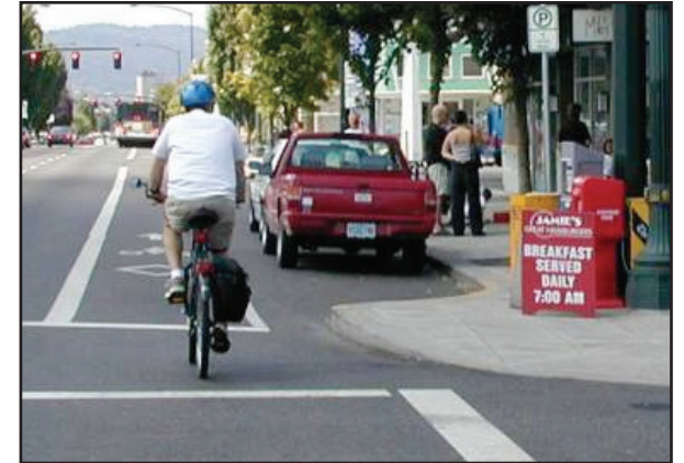
Curb extensions reduce pedestrian crossing distances.
